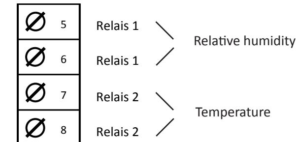
Relay outputs: potential free, normally open
