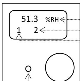
Alternately displays current relative humidity/temperature
