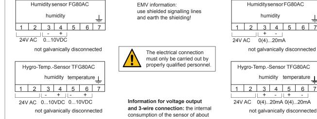
15...25 mA causes a voltage drop on the supply lines. If the measuring signal is taken from terminal 4 / terminal 6 to the connecting point at the power supply (three-wire circuit), then an additional measuring error is incurred, dependant upon the circuit length. A 4-wire connection is recommended.
