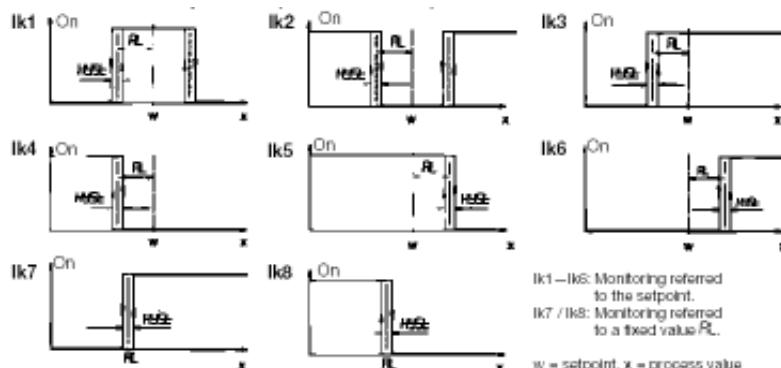
Choose the required limit comparator by pressing **▲** or **▼**. It will be automatically saved after about 2 sec.
